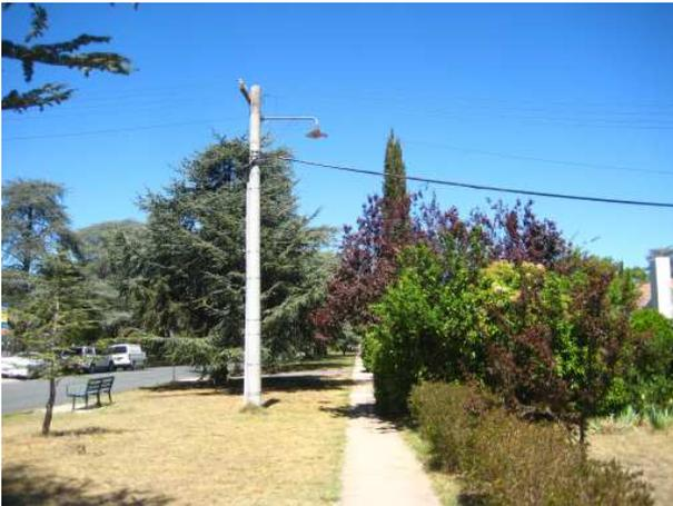
“Street” light correctly positioned to light the footpath, not the street
